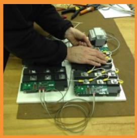
Connection of the Power Electronic FCL prototype
