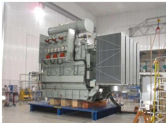
Figure 2-9: FCL side view with AC cable box
