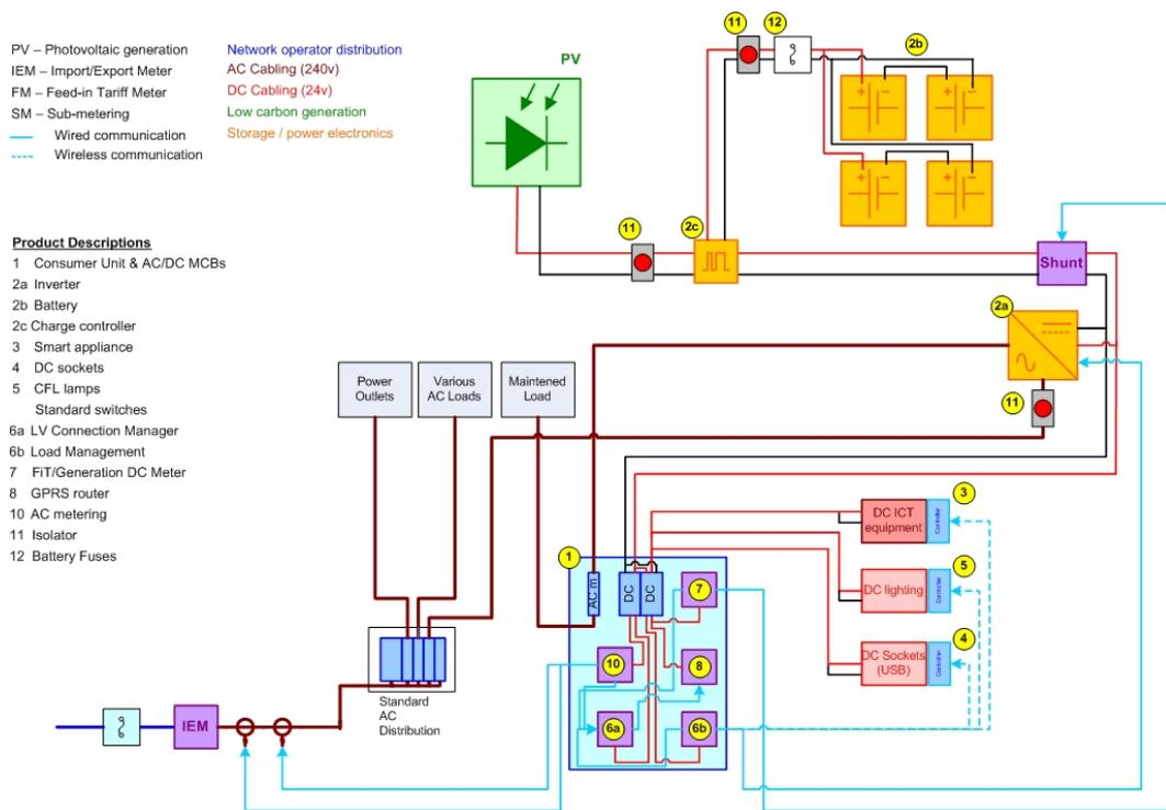
Figure 5 - Typical AC/DC system connections
