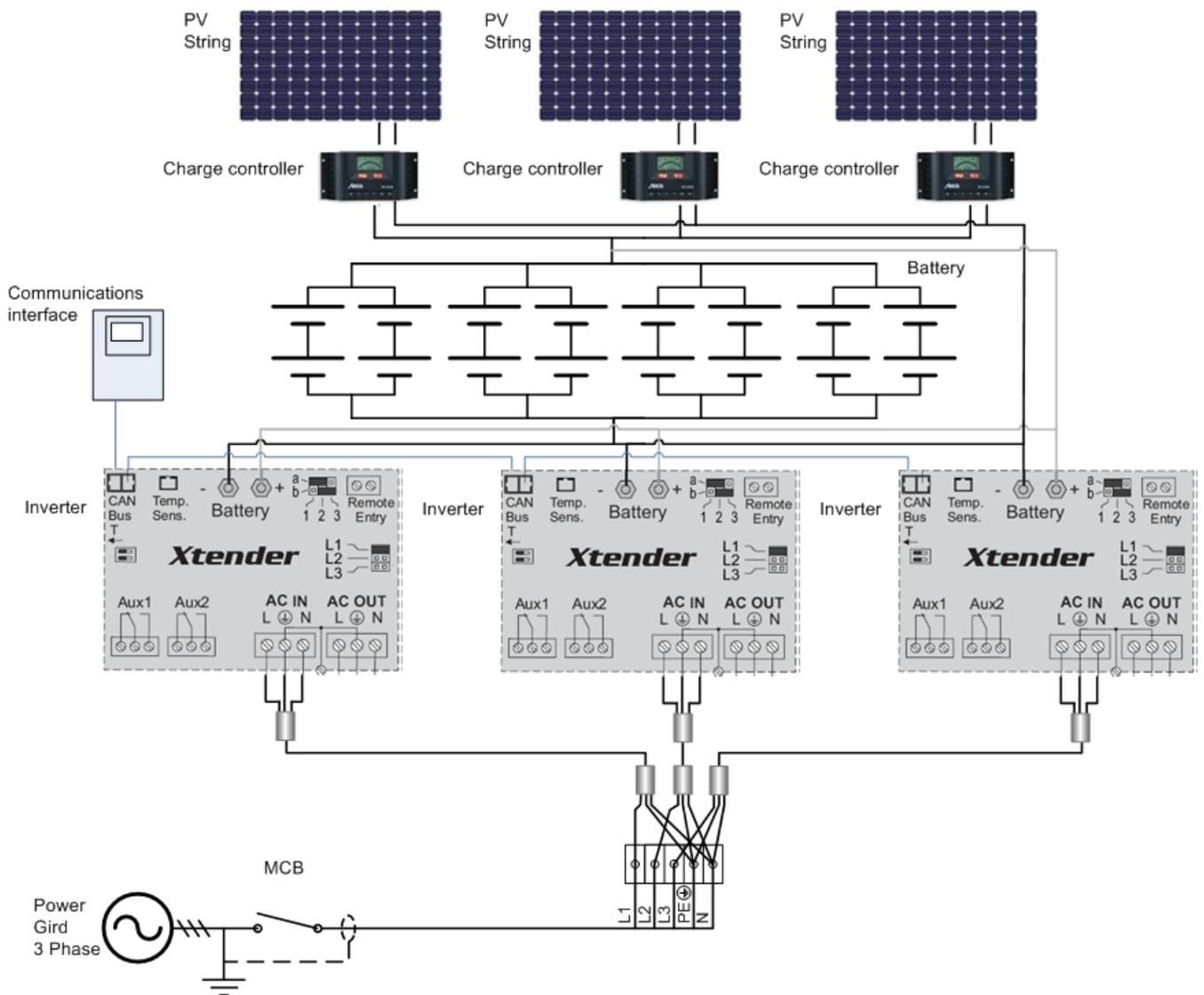
Figure 11 - Typical 3 phase Inverter connections
