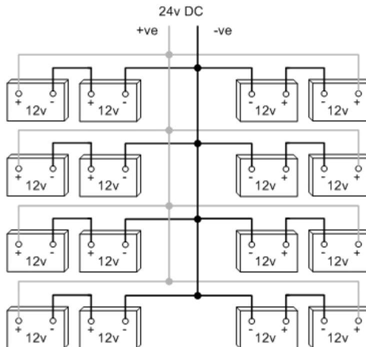
**Figure 12 - Battery Connections**
