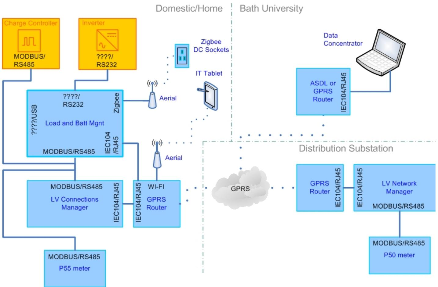
Figure 8 - Domestic Communications Detailed Architecture
