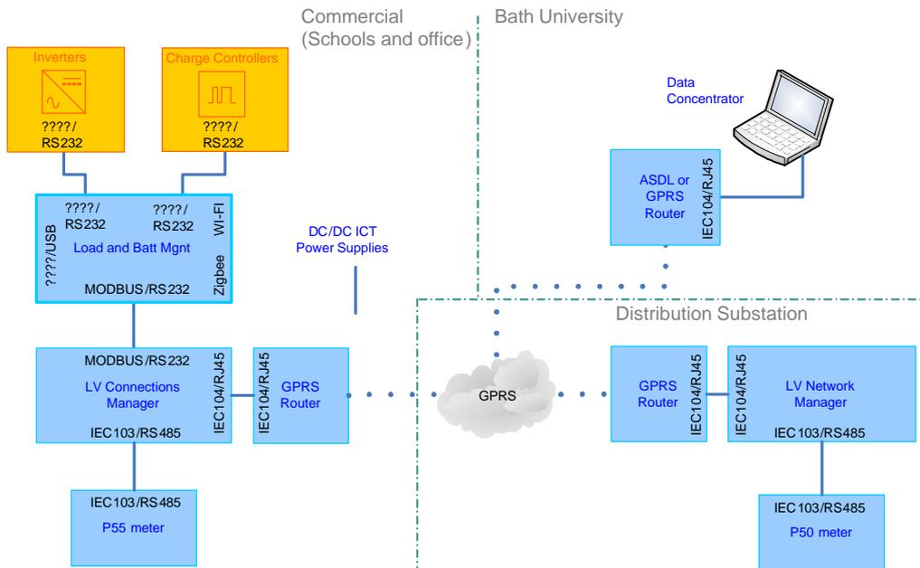
**Figure 15 - Commercial properties Communications Detailed Architecture**
