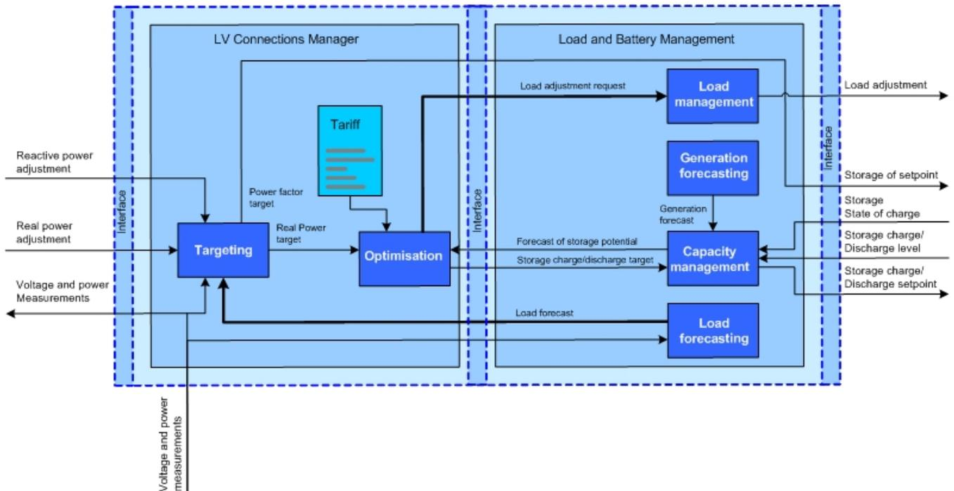
**Figure 2 - Dataflow and Functions contain within the LV Connection Manager & Load and Battery Manager**
