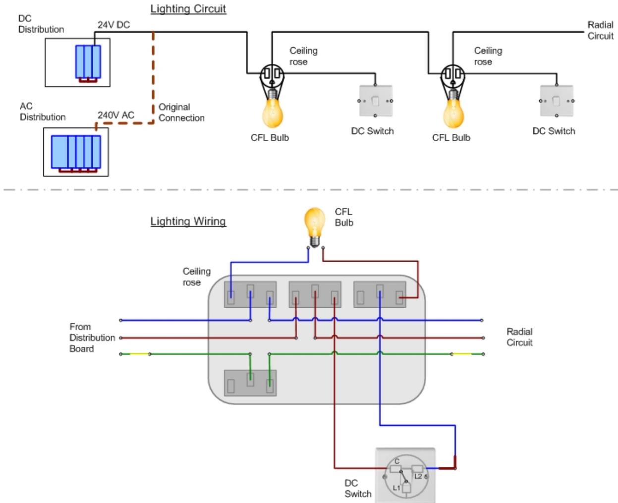
**Figure 6 - Lighting system connections**
