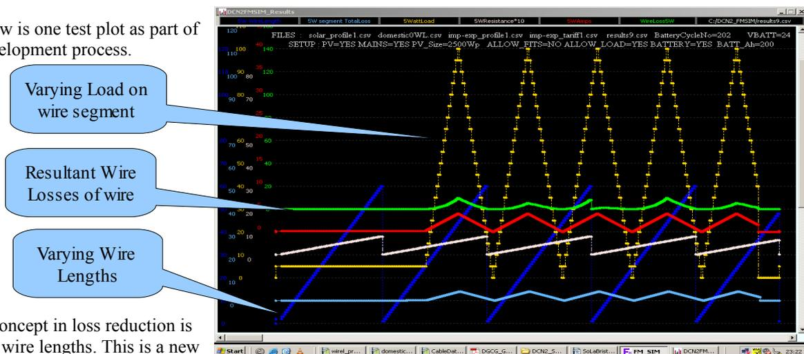
A new concept in loss reduction is Varying wire lengths. This is a new concept for fixed domestic wiring system. This is concept exploration only. The main tool however, can and does provide segment based losses for installation.
