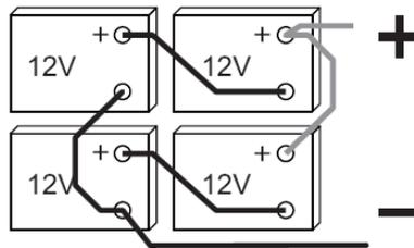
**Figure 4 - Battery Connections.**
