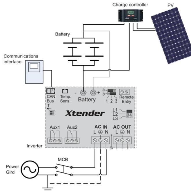
**Figure 3 - Typical Inverter connections**
