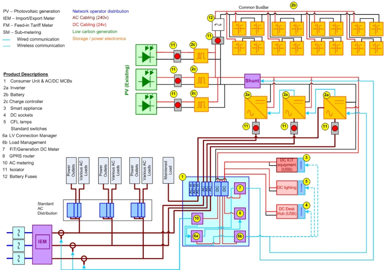
Figure 13 - Typical AC/DC system connections
