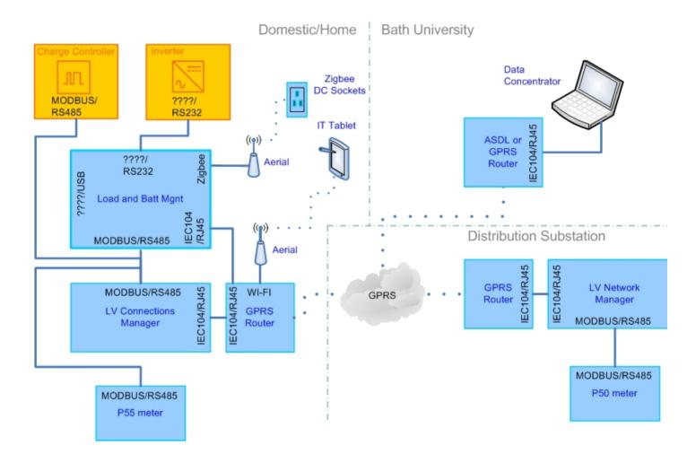
Figure 8 - Domestic Communications Detailed Architecture
