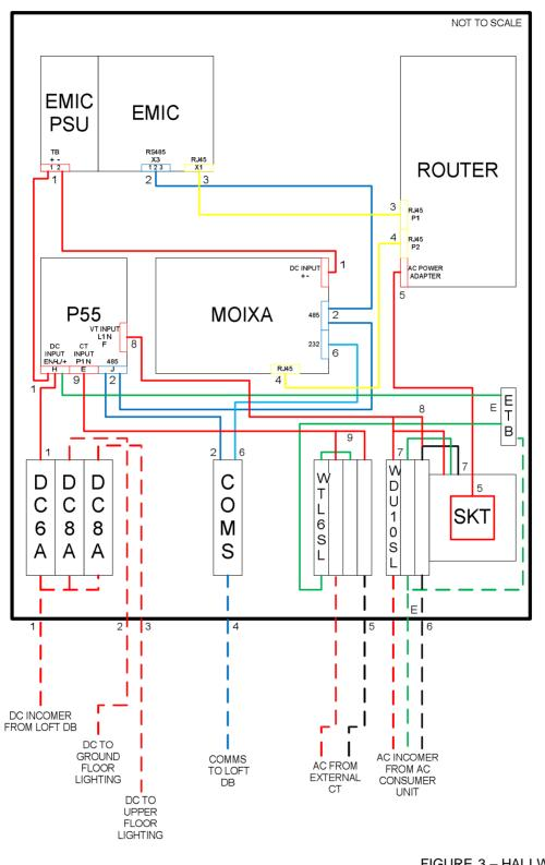
FIGURE 3 – HALLWAY; CABLE CONNECTION REQUIREMENTS
