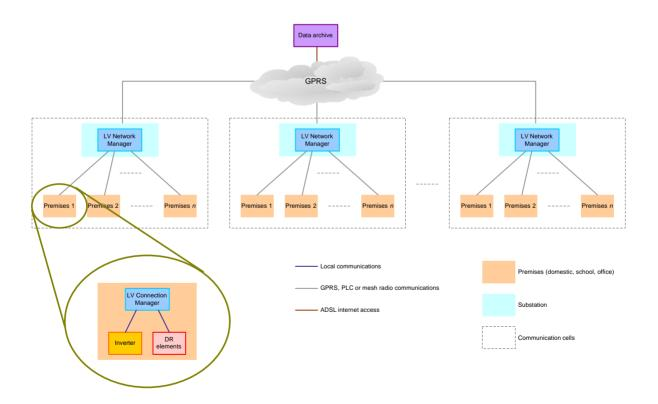
Figure 7 - Overall Communications Architecture
