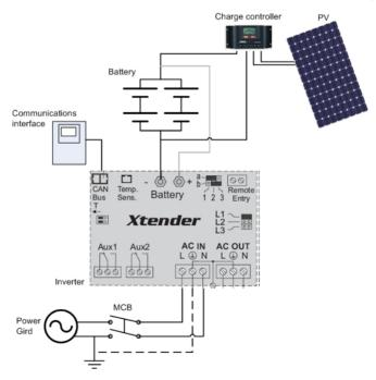
Figure 3 - Typical Inverter connections
