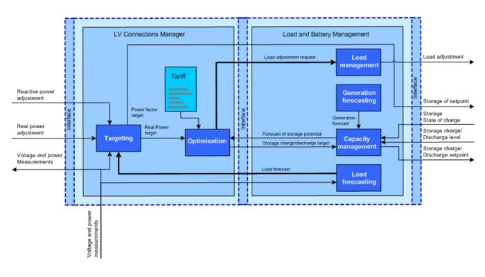
Figure 2 - Dataflow and Functions contain within the LV Connection Manager & Load and Battery Manager
