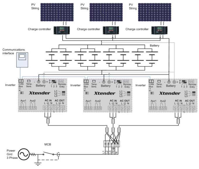
Figure 11 - Typical 3 phase Inverter connections
