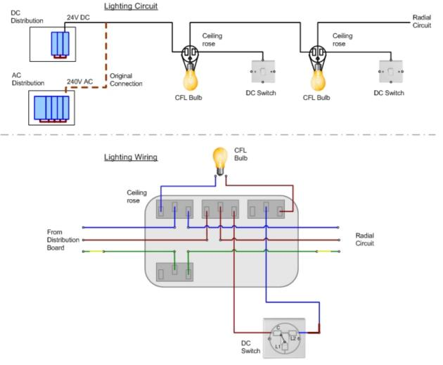
Figure 6 - Lighting system connections
