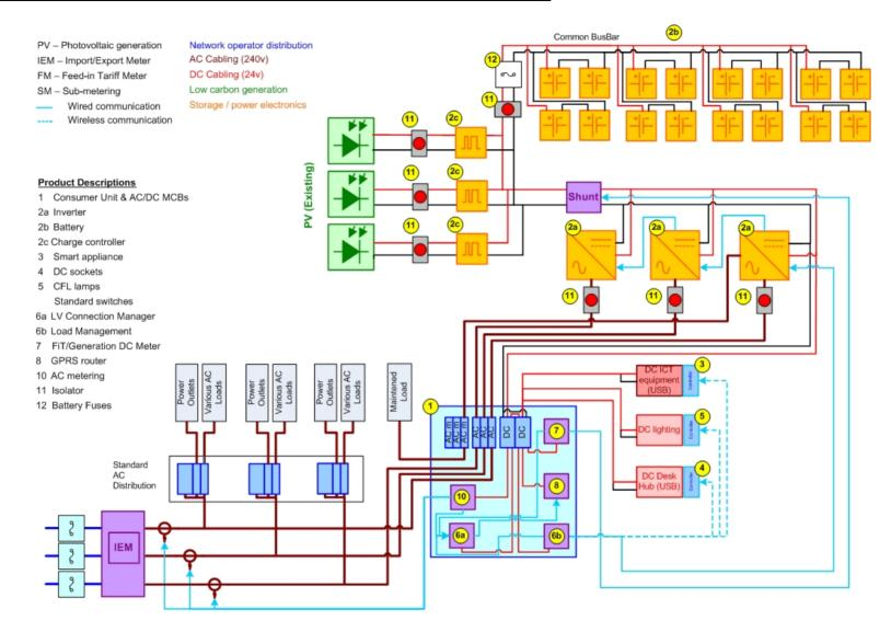
Figure 13 - Typical AC/DC system connections
