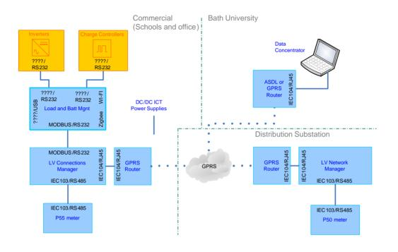
Figure 15 - Commercial properties Communications Detailed Architecture
