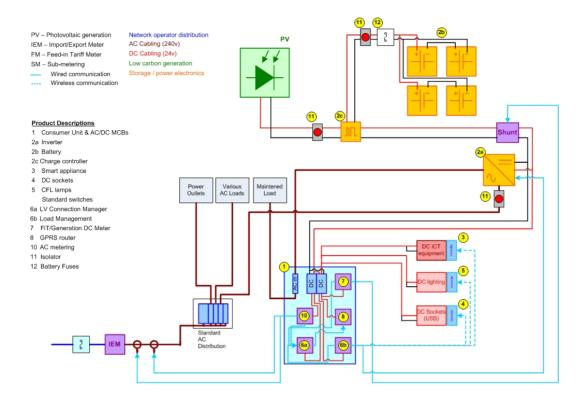
Figure 5 - Typical AC/DC system connections
