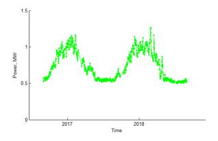
Figure 73 Long term mean daily feeder demand (Wavendon Gate Local HV feeder)
