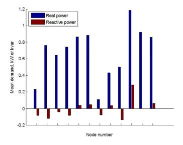
Figure 15 Mean demand for meter connections on Pilot LV feeder
