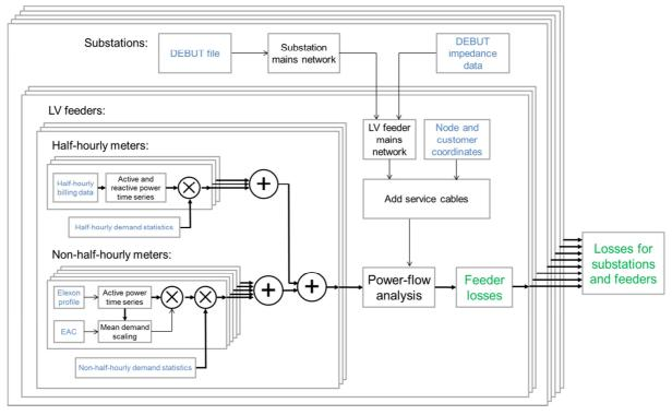
Figure 21 Outline of LV feeder loss assessment method
