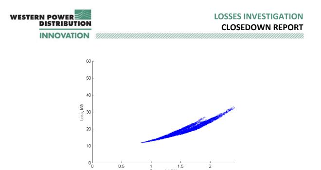
Figure 48 Sample monitored HV feeder loss vs load plot, 1 minute loss/load points using I<sup>2</sup>R calculation method
