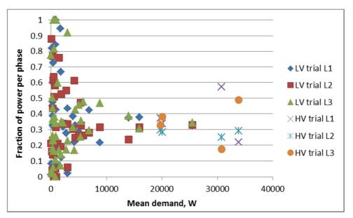
Figure 163 Mean unbalance of three-phase meters
