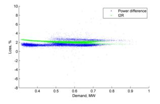
Figure 108 Aug 2017 Loss, % vs demand (Wolverton HV feeder)
