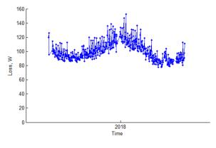
Figure 118 Long term mean daily (I<sup>2</sup>R) loss (Ramsey Dom. LV feeder)
