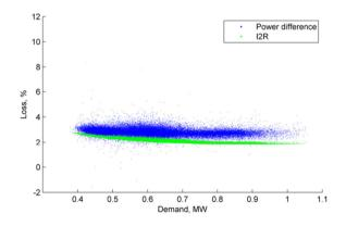
Figure 104 Jul/Aug 2017 Loss, % vs demand (Silver End HV feeder)
