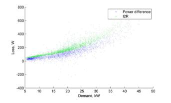
Figure 151 Jan 2018 Loss, kW vs demand, 10 min. av. (Ramsey OH LV feeder)
