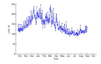
Figure 150 Long term mean daily (I<sup>2</sup>R) loss (Ramsey OH LV feeder)
