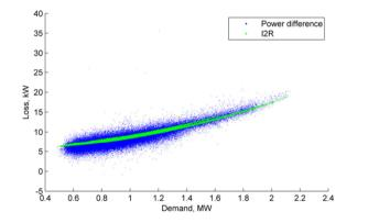
Figure 75 Mar 2018 Loss, kW vs demand (Wavendon Gate Local HV feeder)
