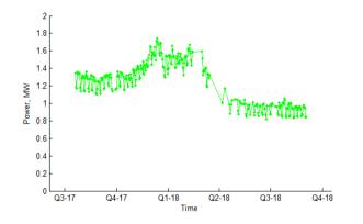
Figure 93 Long term mean daily feeder demand (The Avenue HV feeder)
