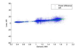
Figure 87 Aug 2018 Loss, kW vs demand (Amway Tongwell HV feeder)
