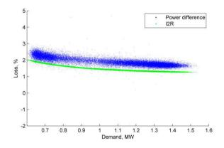
Figure 100 Aug 2018 Loss, % vs demand (Riverside Park HV feeder)
