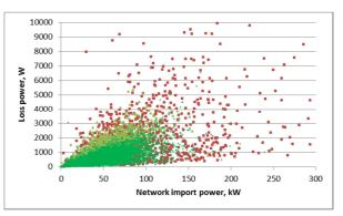
Figure 45 LV feeder loss assessment results, with potentially unreliable results highlighted
