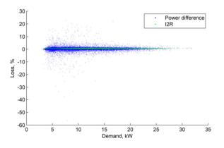
Figure 112 Jan 2018 2017 Loss, % vs demand, 1 min. av. (Dom. Pilot LV feeder)
