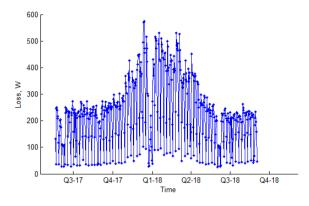
Figure 138 Long term mean daily (I<sup>2</sup>R) loss (Braddan I&C LV feeder)
