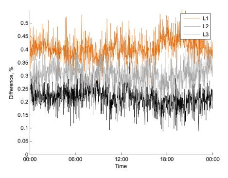
Figure 11 Difference between calculated and measured Distribution Substation voltage on Woodlands feeder, 28<sup>th</sup> March 2016
