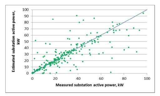
Figure 172 Mean demand from loss assessment and measurement for HV trials feeders
