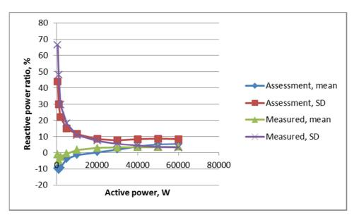
Figure 174 Mean and standard deviation of reactive power for domestic feeders at Milton Keynes trial distribution substations, from measured data and from loss assessment method
