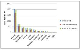
Figure 42 Loss results comparison for monitored LV feeders
