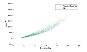
Figure 123 Jan 2018 Loss, kW vs demand, 10 min. av. (Tromode Dom. LV feeder)
