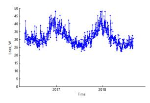
Figure 110 Long term mean daily (I<sup>2</sup>R) loss (Domestic Pilot LV feeder)
