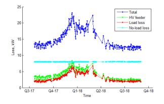
Figure 94 Long term mean daily (I<sup>2</sup>R) loss (The Avenue HV feeder)
