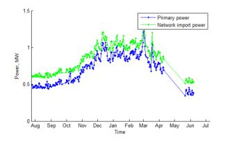
Figure 101 Long term mean daily feeder demand (Silver End HV feeder)
