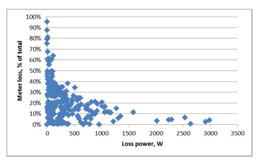
Figure 64 Metering loss as a proportion of the total loss power for LV feeders in Milton Keynes trial.
