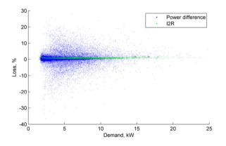
Figure 144 Aug 2018 Loss, % vs demand, 1 min. av. (Santon OH LV feeder)
