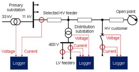
Figure 1 Schematic of HV feeder monitoring
