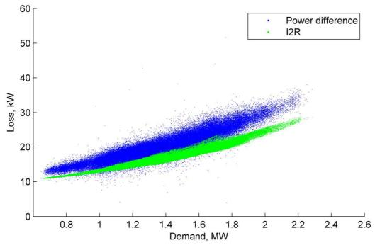
Figure 16 Loss vs demand for 1-minute samples on Woodlands HV feeder
