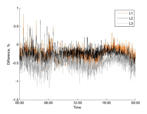
Figure 10 Difference between calculated and measured substation current, 28<sup>th</sup> March 2016
