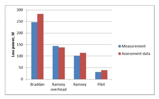
Figure 171 Mean loss power for LV trials feeders with demand and network approximations
