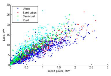
Figure 54 Transformer no-load loss vs. import power
