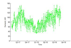
Figure 129 Long term mean daily feeder demand (Peel B I&C LV feeder)
