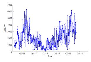
Figure 130 Long term mean daily (I<sup>2</sup>R) loss (Peel B I&C LV feeder)
