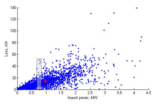
Figure 51 Loss vs. network import power for HV feeders showing mean feeder loss-load point in red
