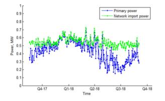
Figure 105 Long term mean daily feeder demand (Wolverton HV feeder)
