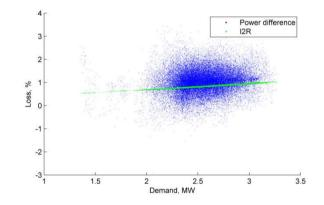
Figure 84 Aug 2018 Loss, % vs demand (Crawley Road Tee Howard Way HV feeder)
