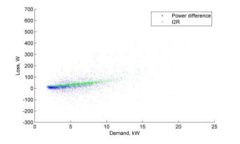
Figure 143 Aug 2018 Loss, kW vs demand, 10 min. av. (Santon OH LV feeder)
