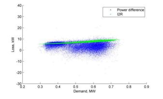
Figure 91 Aug 2018 Loss, kW vs demand (Ackerman Tongwell Aldrich Drive Tee HV feeder)
