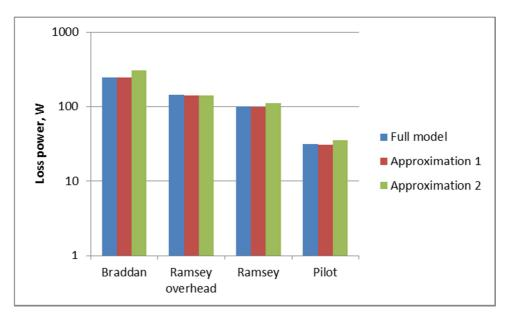
Figure 169 Impact of service cable approximations on LV trials feeders
