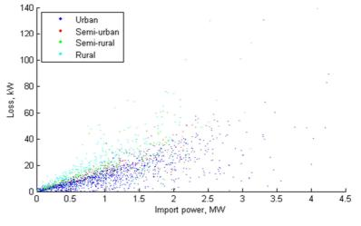
Figure 53 Loss vs. network import power coloured for feeder type
