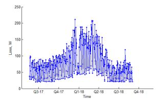
Figure 134 Long term mean daily (I<sup>2</sup>R) loss (Ballasalla I&C LV feeder)
