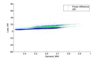
Figure 107 Aug 2017 Loss, kW vs demand (Wolverton HV feeder)
