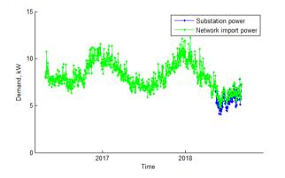
Figure 109 Long term mean daily feeder demand (Domestic Pilot LV feeder)
