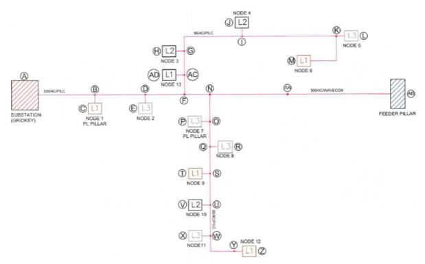
Figure 9 Pilot LV feeder
