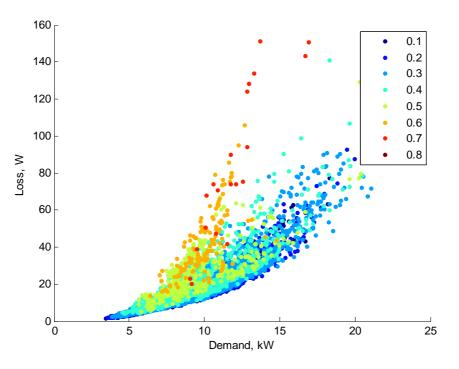
Figure 35 Loss vs. demand with colour indicating unbalance factor
