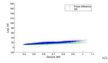
Figure 103 Jul/Aug 2017 Loss, kW vs demand (Silver End HV feeder)
