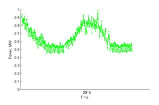
Figure 89 Long term mean daily feeder demand (Ackerman Tongwell Aldrich Drive Tee HV feeder)
