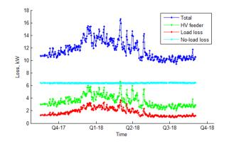
Figure 106 Long term mean daily (I<sup>2</sup>R) loss (Wolverton HV feeder)
