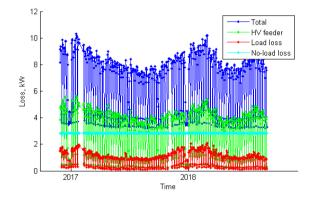
Figure 86 Long term mean daily (I<sup>2</sup>R) loss (Amway Tongwell HV feeder)
