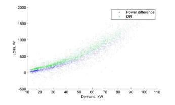
Figure 115 Jan 2018 Loss, kW vs demand, 10 min. av. (Laxey Dom. LV feeder)
