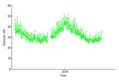
Figure 34 Trend data for Dom#1 LV Feeder (to August 2018)
