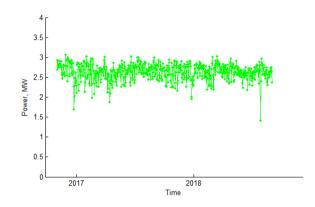
Figure 81 Long term mean daily feeder demand (Crawley Road Tee Howard Way HV feeder)
