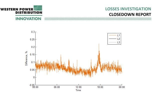
Figure 13 Difference between calculated and measured substation voltages for a load on phases L1
