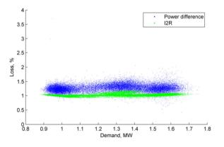
Figure 96 Sep 2017 Loss, % vs demand (The Avenue HV feeder)
