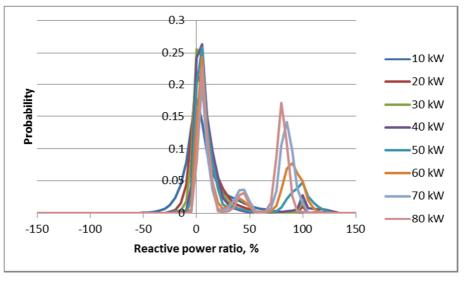
Figure 38 Probability distribution of reactive power for LV feeders
