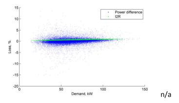
Figure 128 Jan 2018 Loss, % vs demand, 1 min. av. (Peel A I&C LV feeder)
