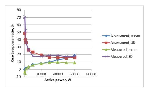
Figure 173 Mean and standard deviation of reactive power for all feeders at Milton Keynes trial distribution substations, from measured data and from loss assessment method
