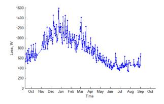
Figure 122 Long term mean daily (I<sup>2</sup>R) loss (Tromode Dom. LV feeder)
