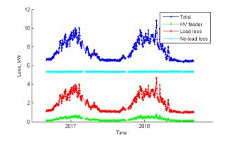
Figure 74 Long term mean daily (I<sup>2</sup>R) loss (Wavendon Gate Local HV feeder)
