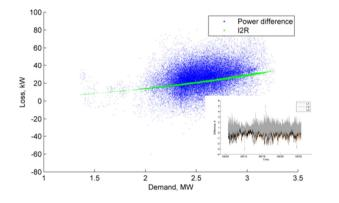
Figure 83 Aug 2018 Loss, kW vs demand (Crawley Road Tee Howard Way HV feeder)
