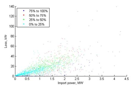
Figure 56 Loss vs. network import power coloured for proportion of losses due to HV cable load losses
