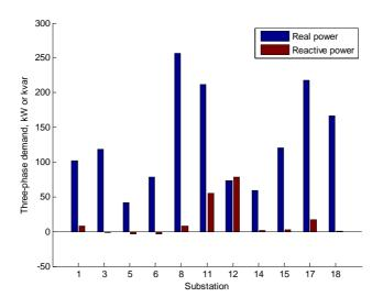
Figure 14 Mean demand for Distribution Substations on Woodlands HV feeder
