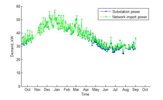
Figure 121 Long term mean daily feeder demand (Tromode Dom. LV feeder)
