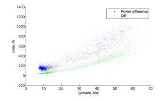
Figure 135 Jan 2018 Loss, kW vs demand, 10 min. av. (Ballasalla I&C LV feeder)
