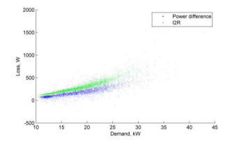
Figure 147 Aug 2018 Loss, kW vs demand, 10 min. av. (Abbeylands OH LV feeder)
