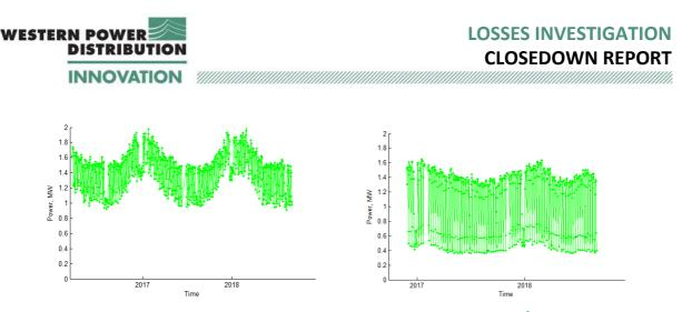
Figure 50 Sample monitored LV feeder loss vs load plot, 1 minute loss/load points using I<sup>2</sup>R calculation method
