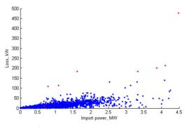
Figure 43 HV feeder loss assessment results, with potentially unreliable results highlighted
