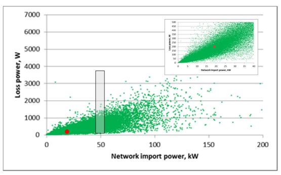
Figure 52 Loss vs. network import power for HV feeders showing mean feeder loss-load point and an indicative trend line
