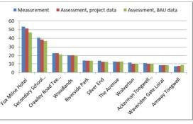
Figure 41 Loss results comparison for monitored HV feeders
