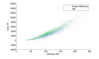
Figure 131 Aug 2018 Loss, kW vs demand, 10 min. av. (Peel B I&C LV feeder)
