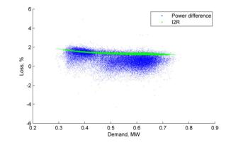
Figure 92 Aug 2018 Loss, % vs demand (Ackerman Tongwell Aldrich Drive Tee HV feeder)
