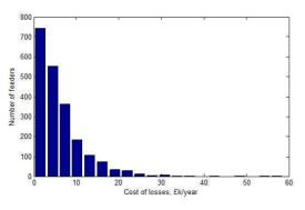
Figure 60 Histogram of number of HV feeders versus annual cost of feeder losses
