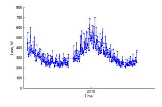
Figure 114 Long term mean daily (I<sup>2</sup>R) loss (Laxey Dom. LV feeder)
