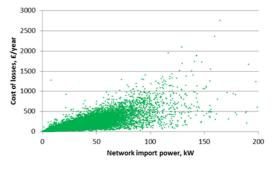
Figure 58 Indicative annual cost of HV feeder technical losses
