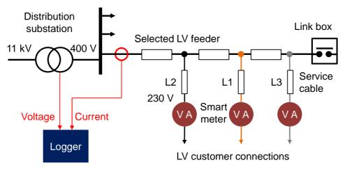
Figure 7 Schematic of LV feeder monitoring
