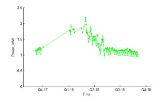
Figure 97 Long term mean daily feeder demand (Riverside Park HV feeder)
