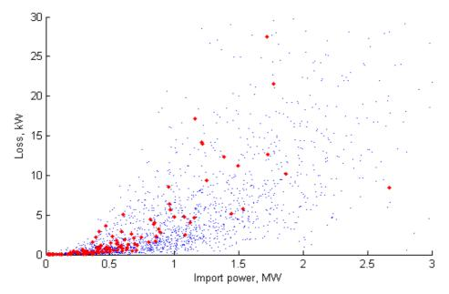
Figure 55 Line loss vs. network import power coloured for voltage (blue: 11 kV, red 6.6 kV)
