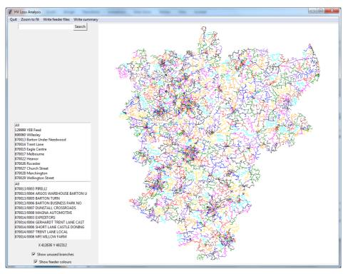
Figure 19 HV loss assessment software Python interface showing East Midlands area feeders
