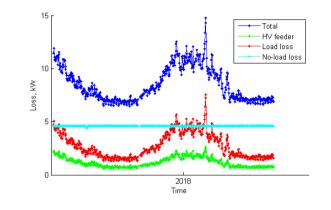
Figure 90 Long term mean daily (I<sup>2</sup>R) loss (Ackerman Tongwell Aldrich Drive Tee HV feeder)
