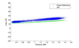
Figure 99 Aug 2018 Loss, kW vs demand (Riverside Park HV feeder)
