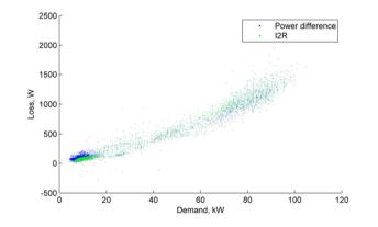
Figure 139 Jan 2018 Loss, kW vs demand, 10 min. av. (Braddan I&C LV feeder)
