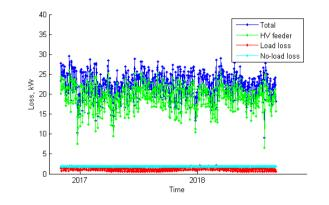
Figure 82 Long term mean daily (I<sup>2</sup>R) loss (Crawley Road Tee Howard Way HV feeder)
