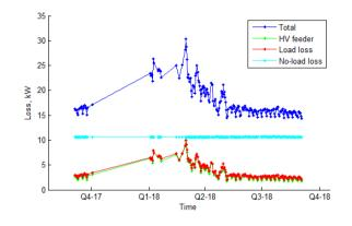
Figure 98 Long term mean daily (I<sup>2</sup>R) loss (Riverside Park HV feeder)
