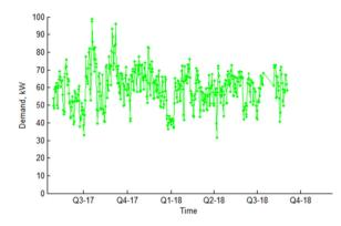
Figure 125 Long term mean daily feeder demand (Peel A I&C LV feeder)
