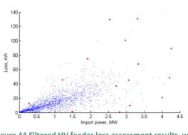
Figure 44 Filtered HV feeder loss assessment results, with outliers highlighted
