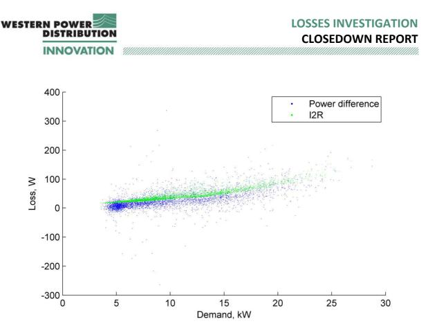
Figure 63 Loss vs demand per 1-minute sample for LV Pilot feeder with 10-minute averaging of the loss results
