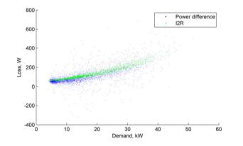
Figure 119 Aug 2018 Loss, kW vs demand, 10 min. av. (Ramsey Dom. LV feeder)
