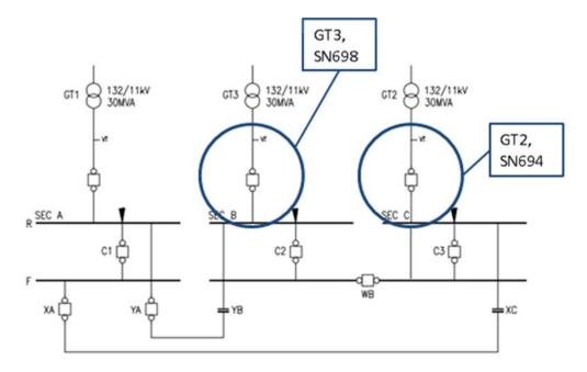
Figure 2-3 - PM7000 logger locations in the Chester Street Primary substation
