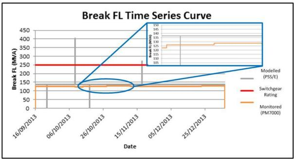
Figure 2-5 - Comparison of modelled and monitored fault level at GT2 in Chester Street Primary substation
