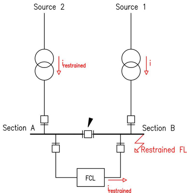
Figure 8-1: An illustrative Primary Substation for fault level reduction calculations
