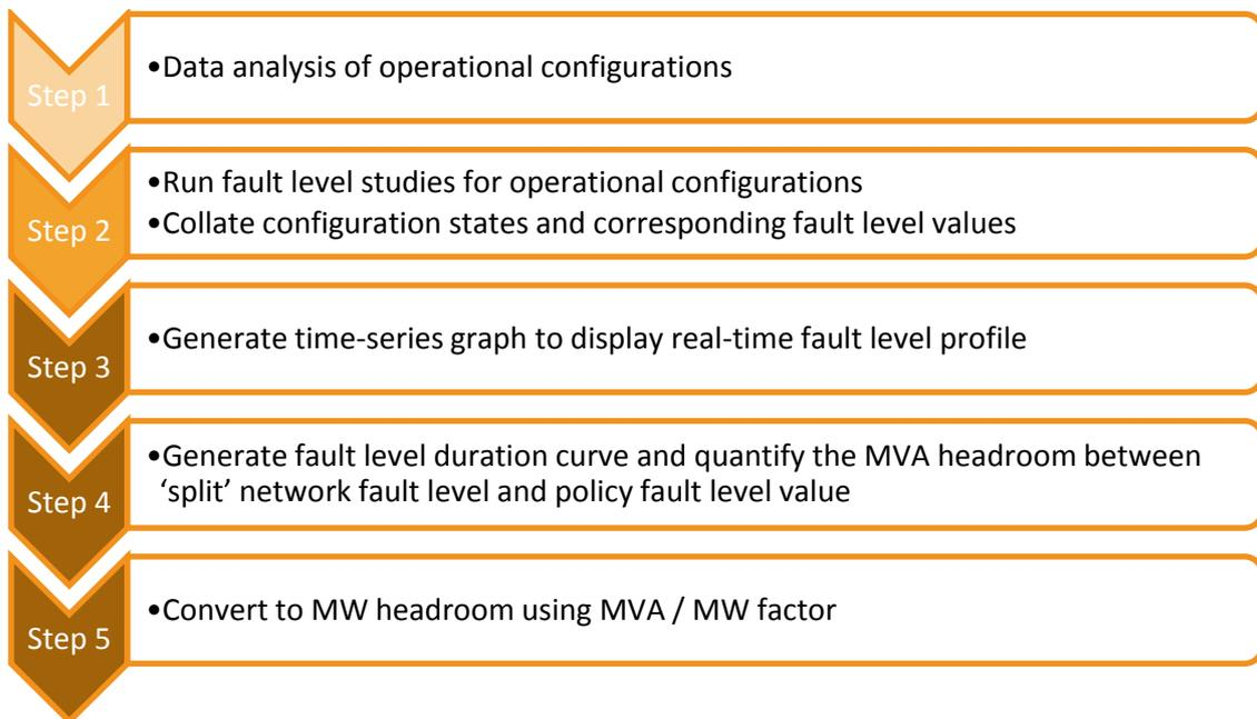
Figure 7-1 Technical analysis of substation fault level profiles
