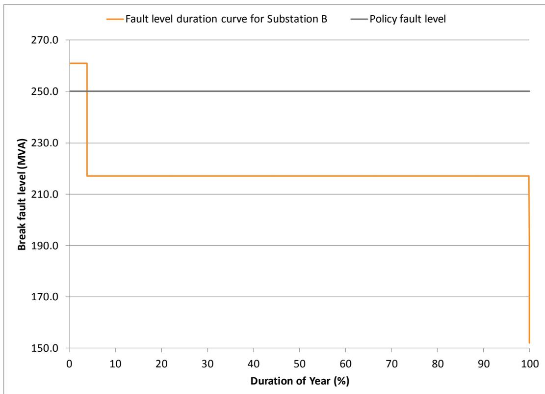
Figure D-6: Fault level duration curve for Substation B for the period 01 September 2012 to 31 August 2013
