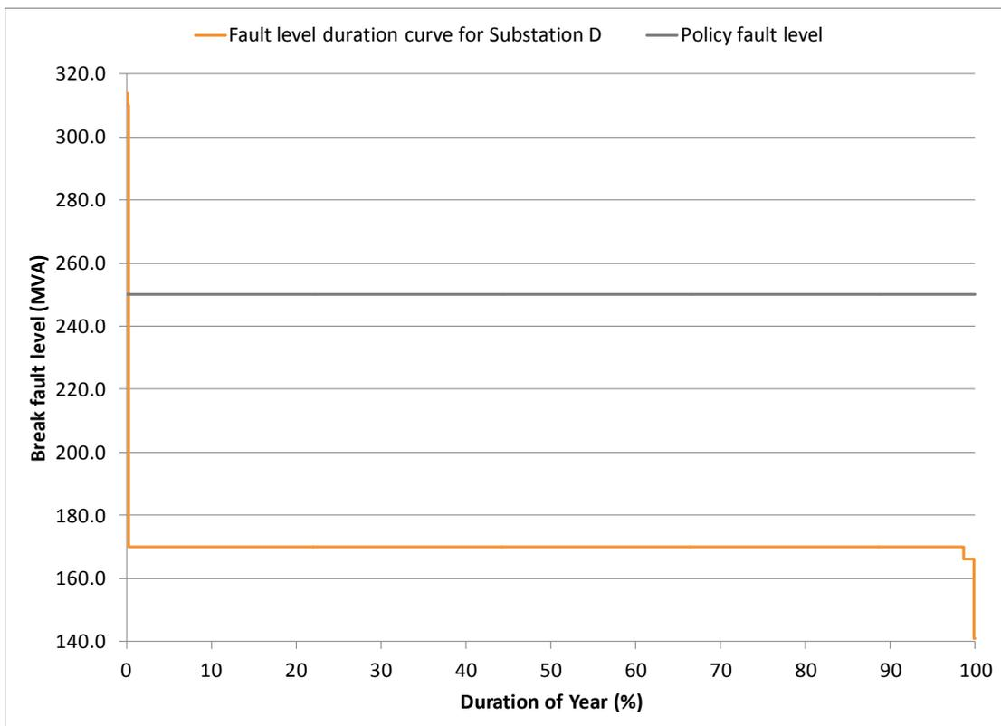
Figure D-12: Fault level duration curve for Substation D for the period 01 September 2012 to 31 August 2013
