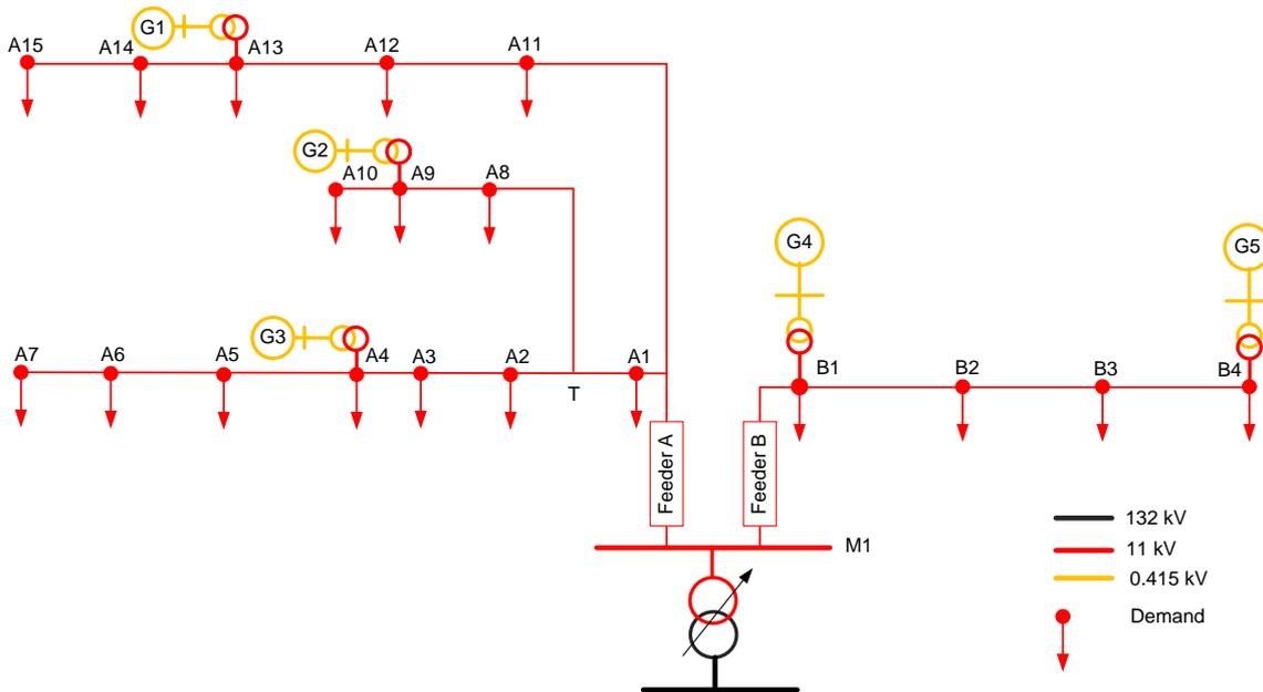
Figure C-1: The sample model representing a short and a long feeder
