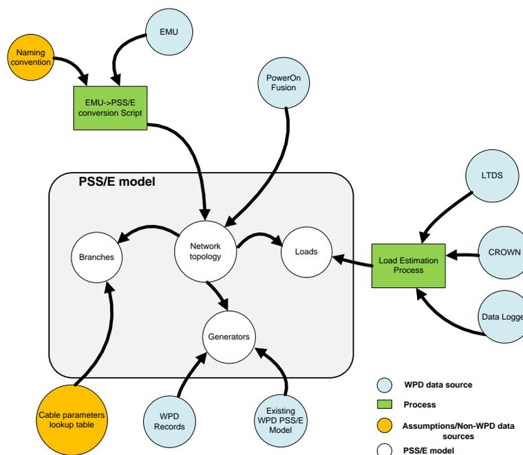
Figure 3-1 Methodology for modelling the HV network in PSS/E
