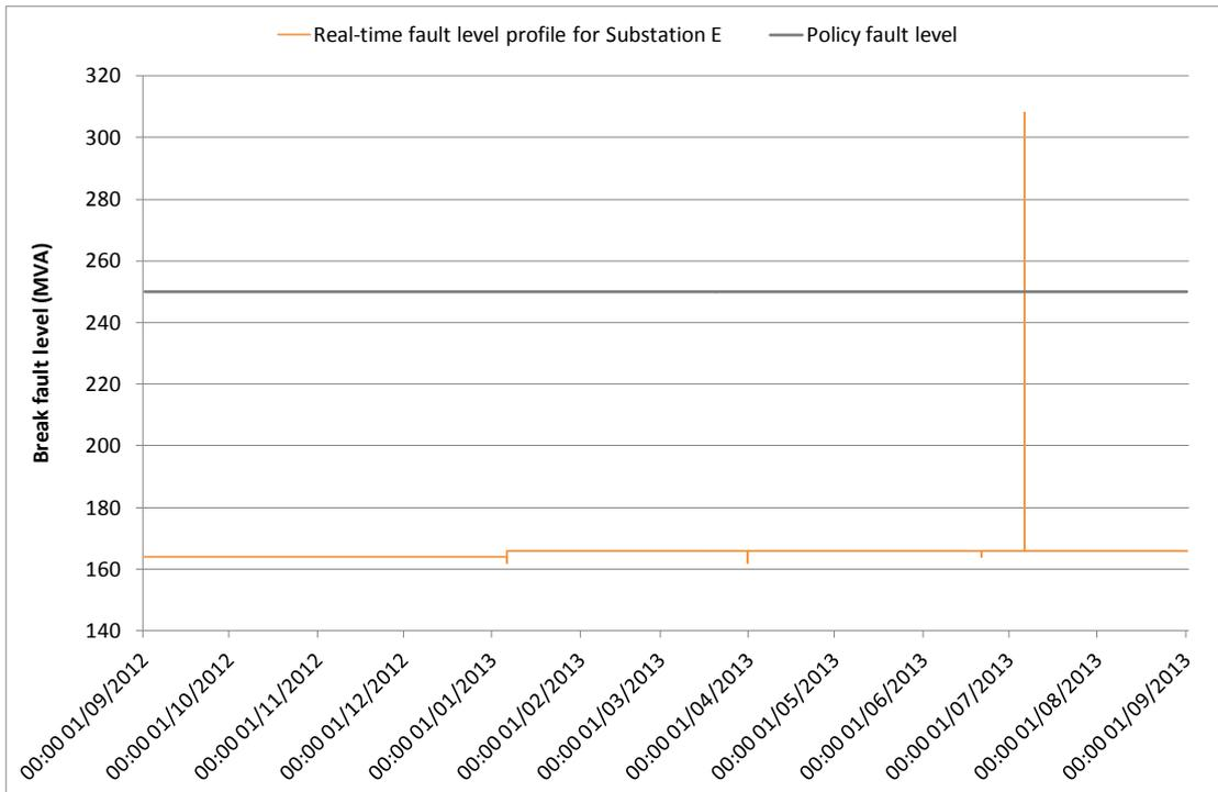
Figure D-14: Real-time fault level profile of Substation E for the period 01 September 2012 to 31 August 2013
