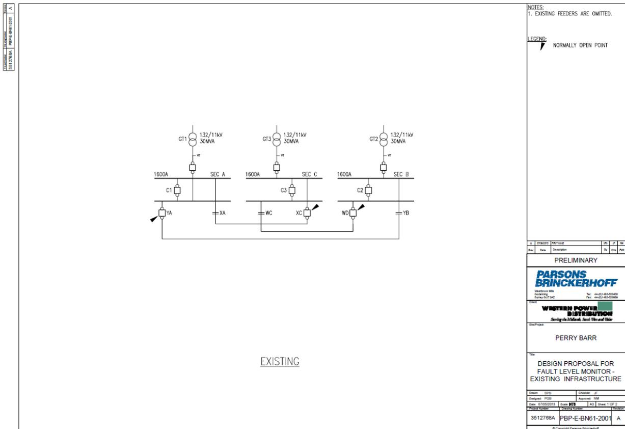
**Figure D-25: Topology of Substation I**
