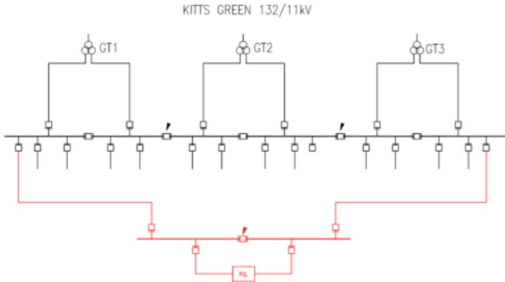
Figure 6-2- Parallel operation with FCL installed within interconnector between GT1 and GT3
