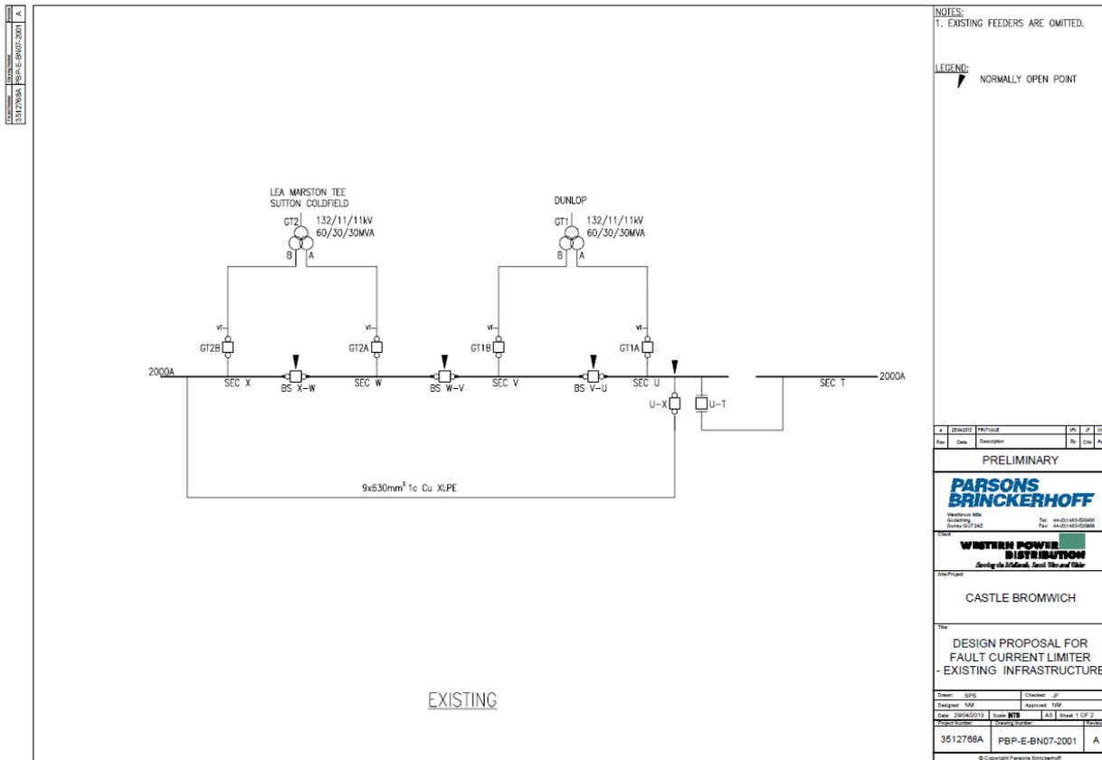
Figure D-4: Topology of Substation B
