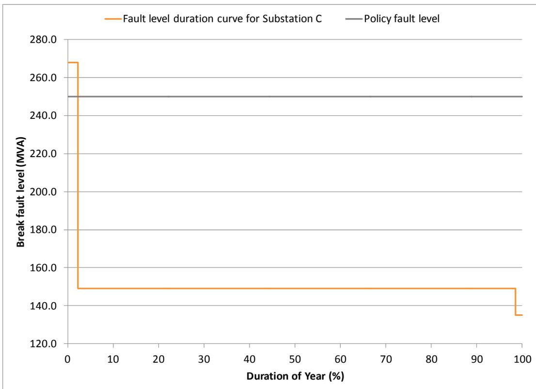
Figure D-9: Fault level duration curve for Substation C for the period 01 September 2012 to 31 August 2013
