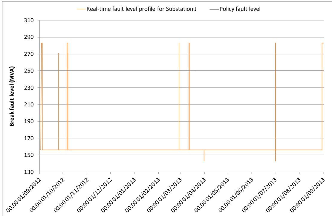
Figure D-29: Real-time fault level profile of Substation J for the period 01 September 2012 to 31 August 2013
