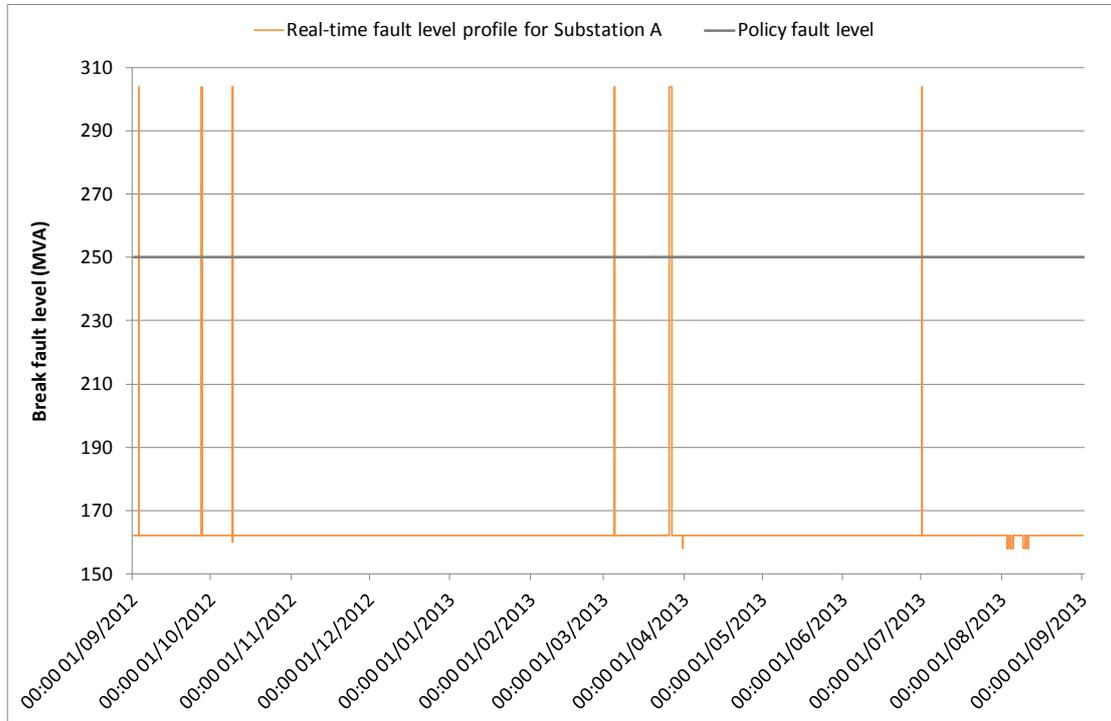
Figure D-2: Real-time fault level profile of Substation A for the period 01 September 2012 to 31 August 2013
