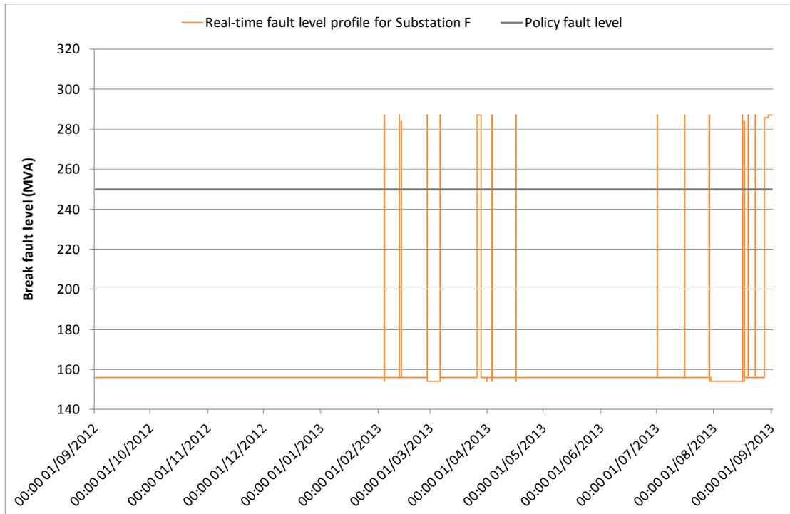
Figure D-17: Real-time fault level profile of Substation F for the period 01 September 2012 to 31 August 2013
