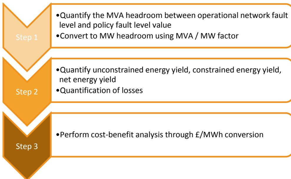
Figure 9-1 Techno-economic analysis of ‘connect and manage’ solution
