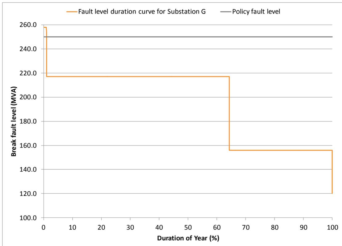
Figure D-21: Fault level duration curve for Substation G for the period 01 September 2012 to 31 August 2013
