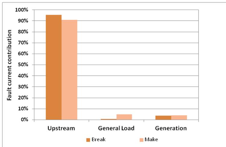
Figure 2-1 – Fault level decomposition into its constituent components with existing generation levels at an illustrative 132kV/11kV Primary Substation
