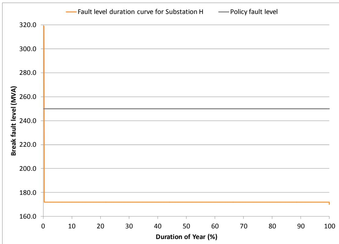
Figure D-24: Fault level duration curve for Substation H for the period 01 September 2012 to 31 August 2013
