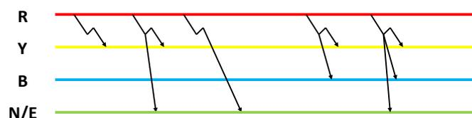
Figure 1-1 - Examples of unintentional conducting paths (faults) in a 3-phase system
