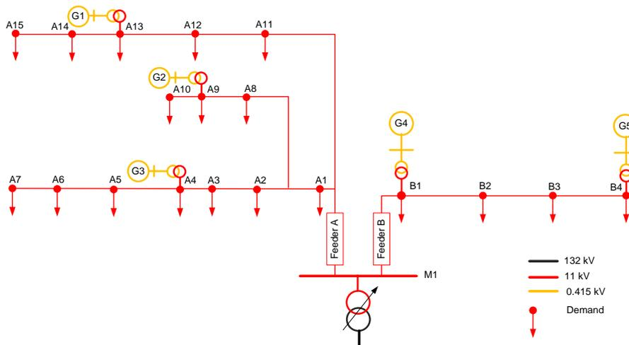
Figure 5-1: The sample model representing a short and a long feeder.
