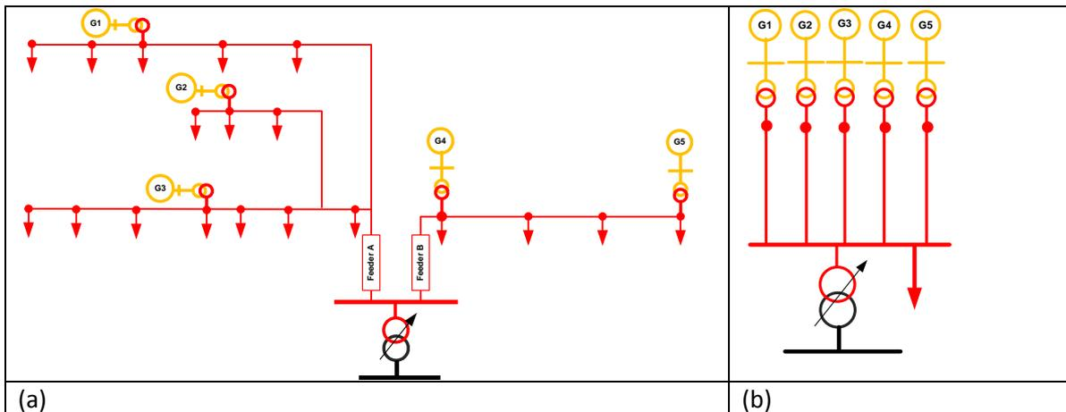
Figure 5-5: Network modelling for connection study (a) a detailed model of 11 kV network (b) an equivalent model of 11 kV network
