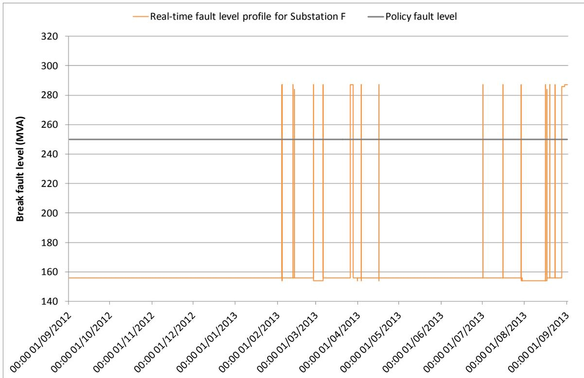
Figure 7-3 – A time series analysis of the real-time fault level profile at Substation F for the period 1 September 2012 – 01 August 2013
