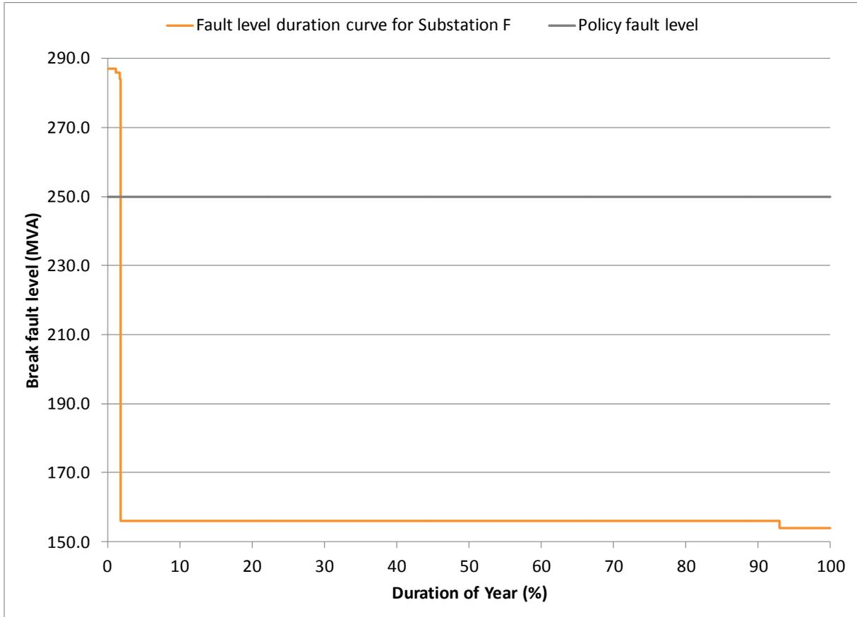
Figure 7-4 – Fault level duration curve for Substation F for the period 01 September 2012 – 31 August 2013
