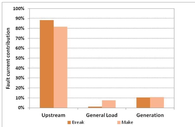
Figure 2-2 – Fault level decomposition into its constituent components with generation penetration levels up to 10% of the firm load capacity of an illustrative 132kV/11kV Primary Substation
