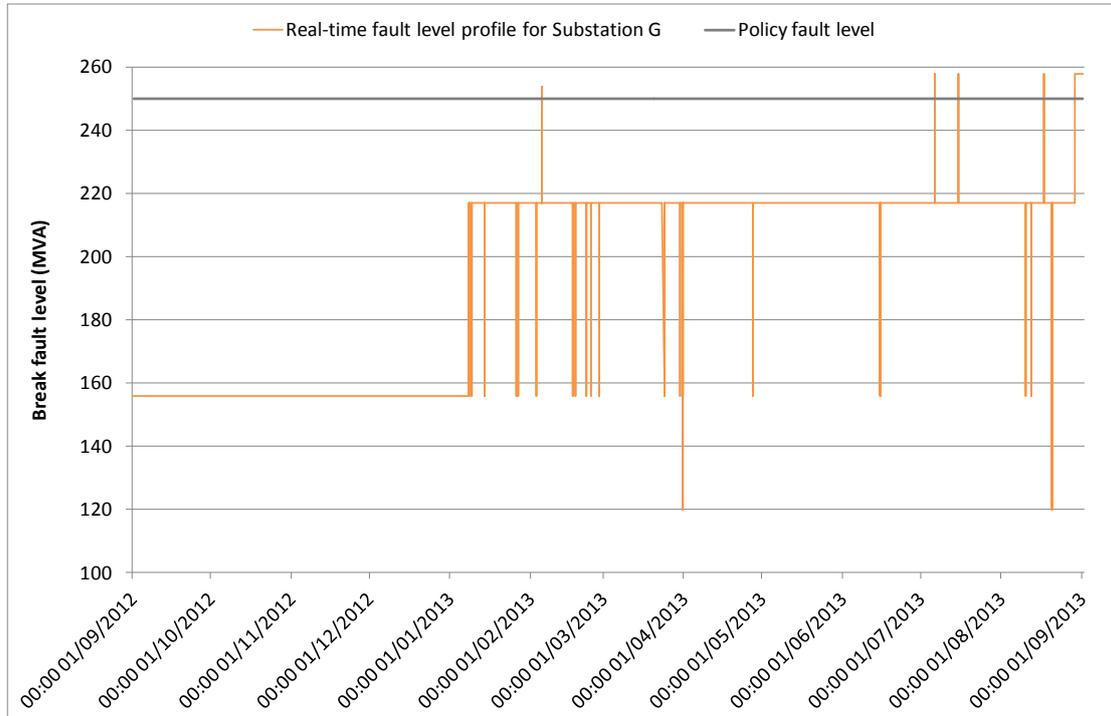
Figure D-20: Real-time fault level profile of Substation G for the period 01 September 2012 to 31 August 2013
