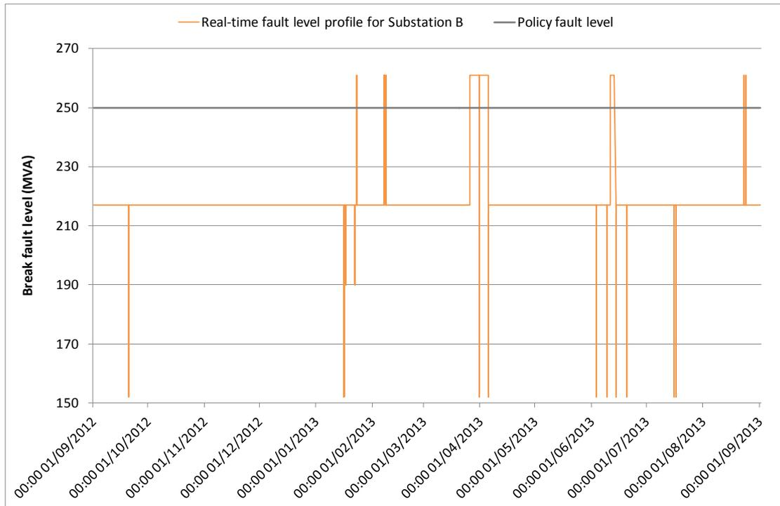
Figure D-5: Real-time fault level profile of Substation B for the period 01 September 2012 to 31 August 2013
