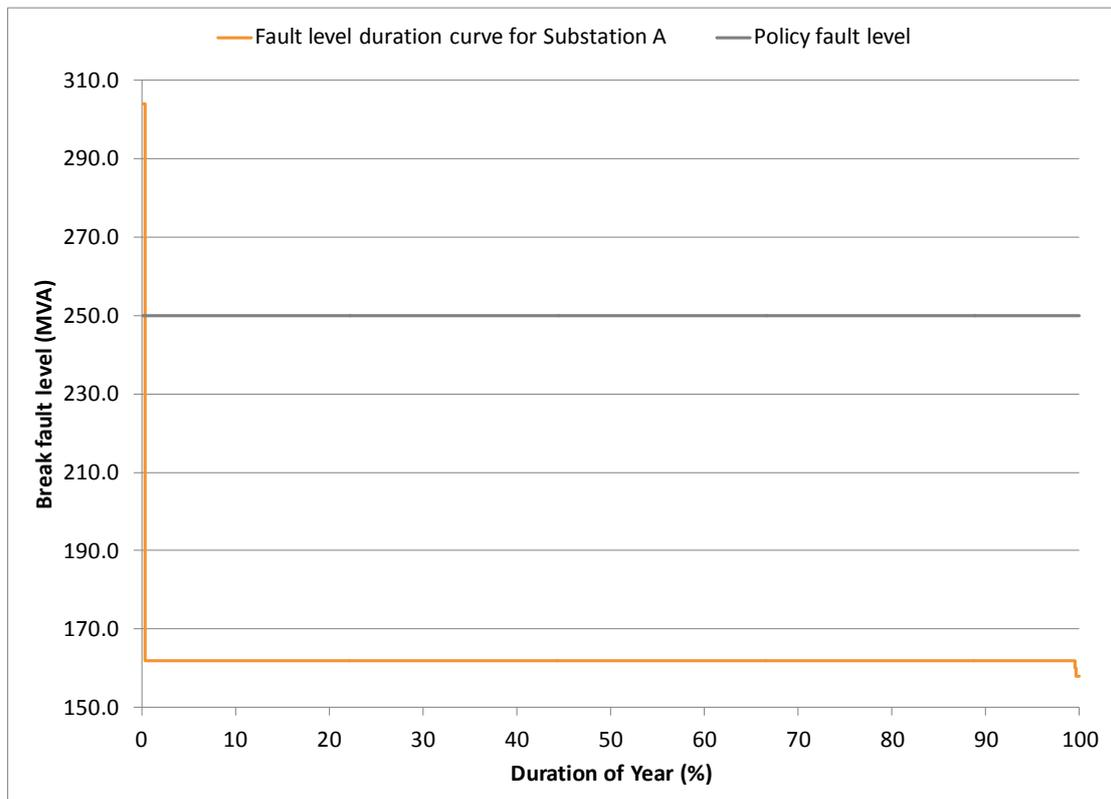
Figure D-3: Fault level duration curve for Substation A for the period 01 September 2012 to 31 August 2013
