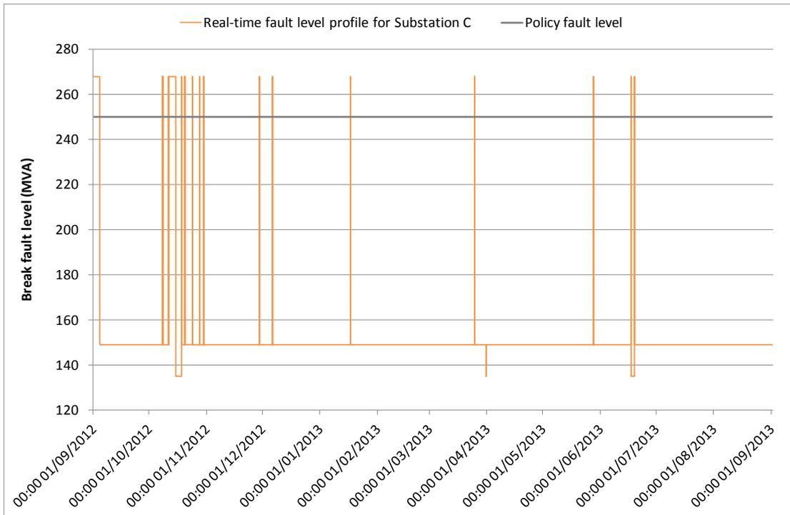
Figure D-8: Real-time fault level profile of Substation C for the period 01 September 2012 to 31 August 2013
