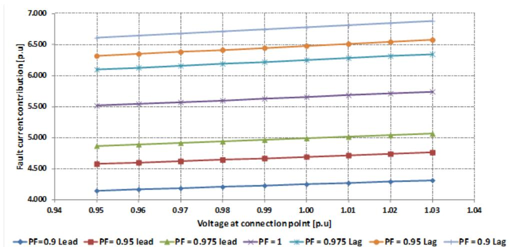
Figure 5-4: The effect of power factor on generator initial rms fault in-feed
