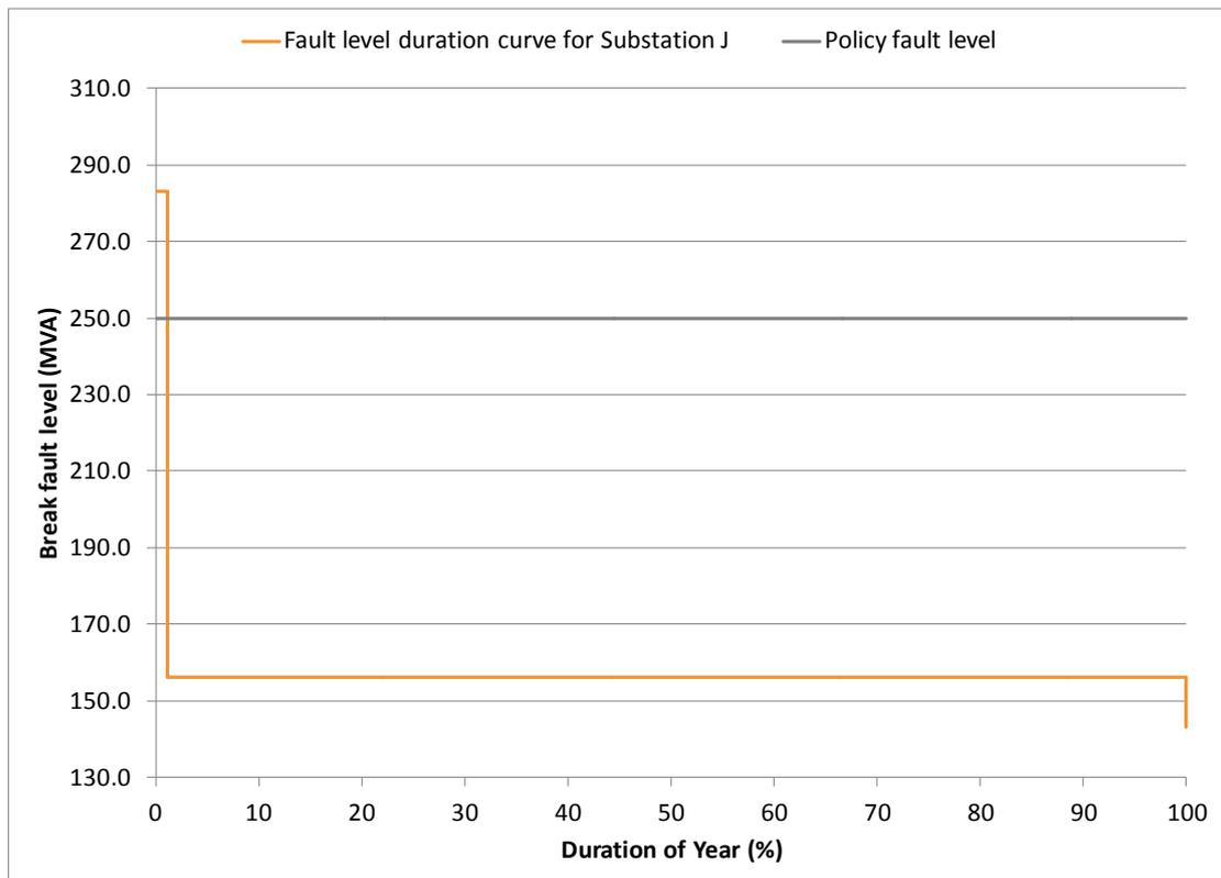
Figure D-30: Fault level duration curve for Substation J for the period 01 September 2012 to 31 August 2013
