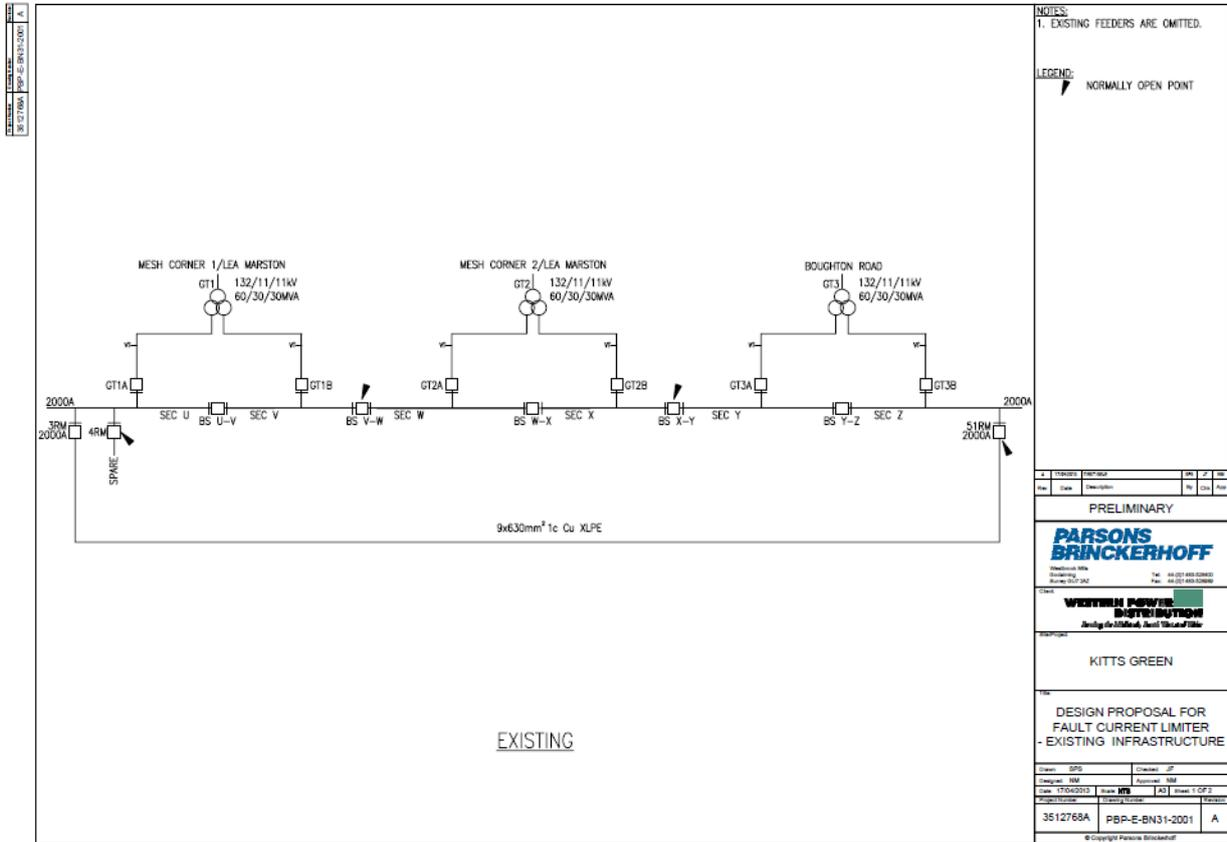
Figure D-1: Topology of Substation A
