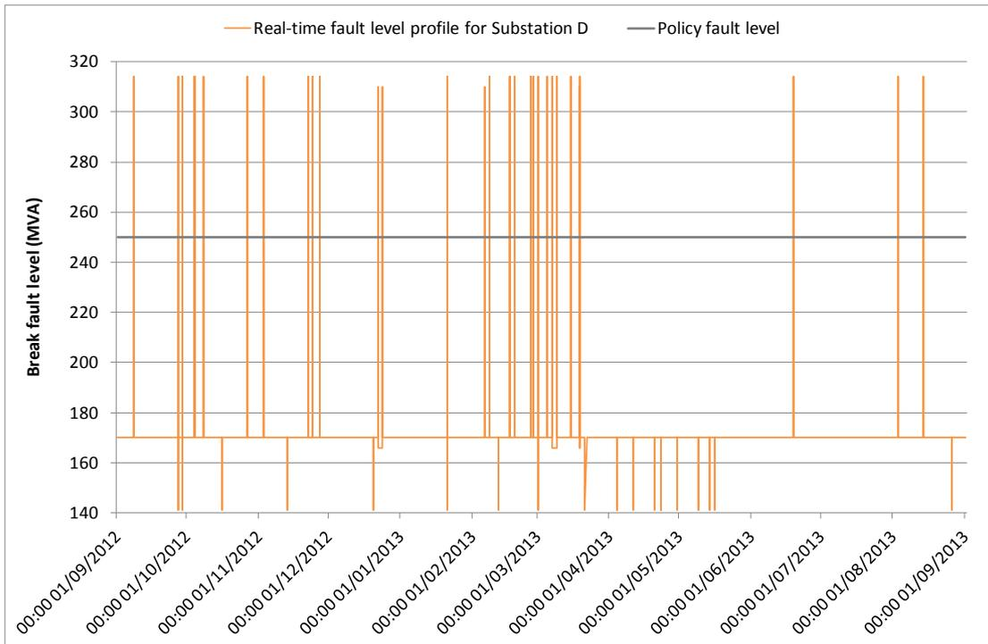
Figure D-11: Real-time fault level profile of Substation D for the period 01 September 2012 to 31 August 2013
