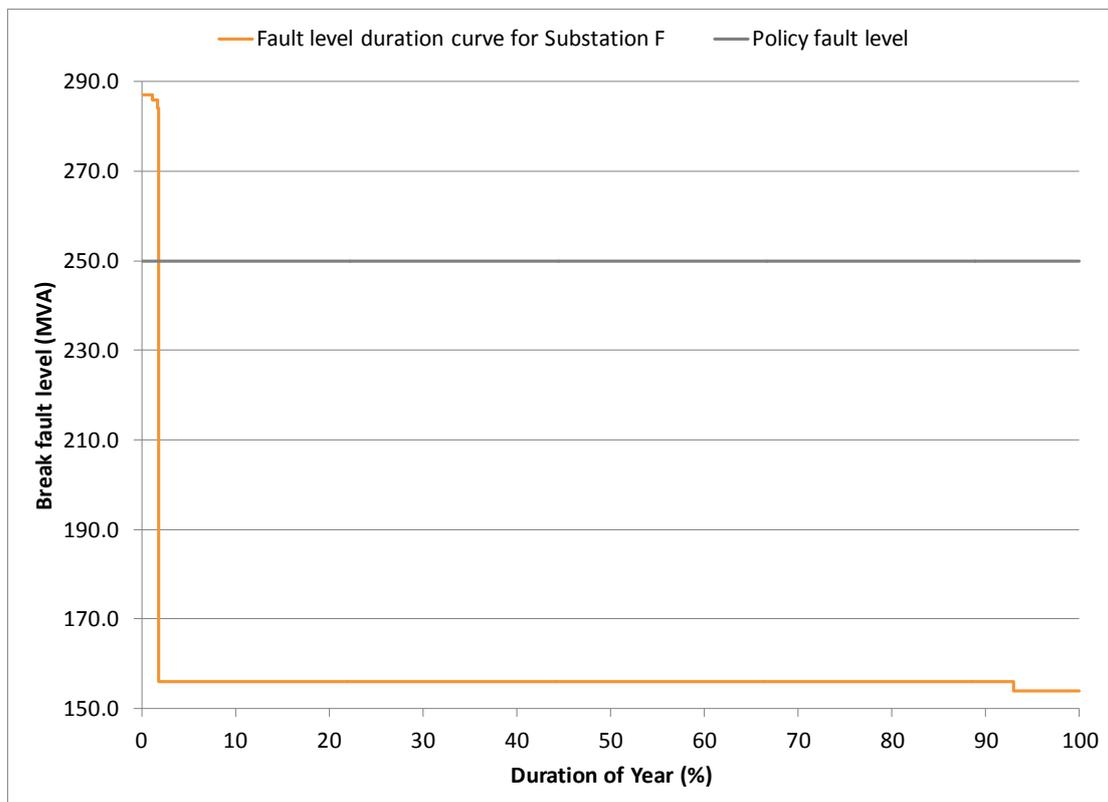
Figure D-18: Fault level duration curve for Substation F for the period 01 September 2012 to 31 August 2013
