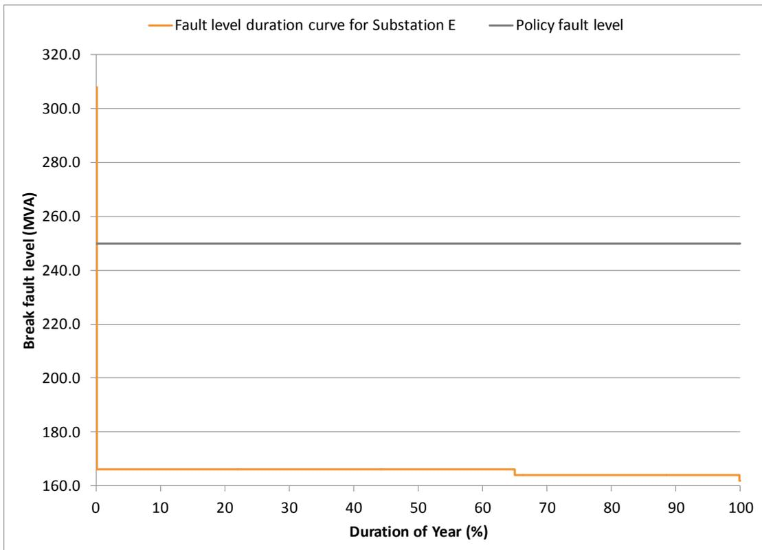
Figure D-15: Fault level duration curve for Substation E for the period 01 September 2012 to 31 August 2013
