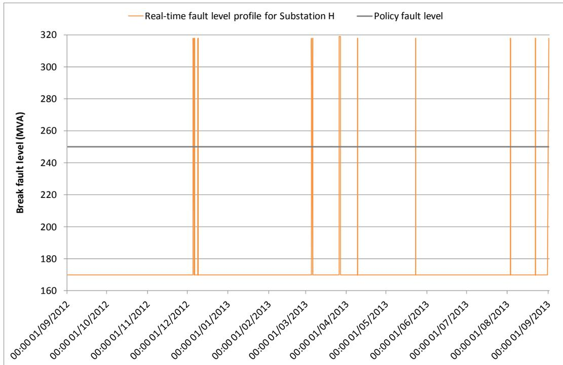
Figure D-23: Real-time fault level profile of Substation H for the period 01 September 2012 to 31 August 2013
