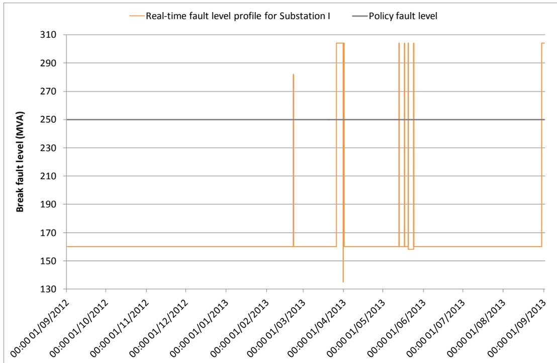
Figure D-26: Real-time fault level profile of Substation I for the period 01 September 2012 to 31 August 2013
