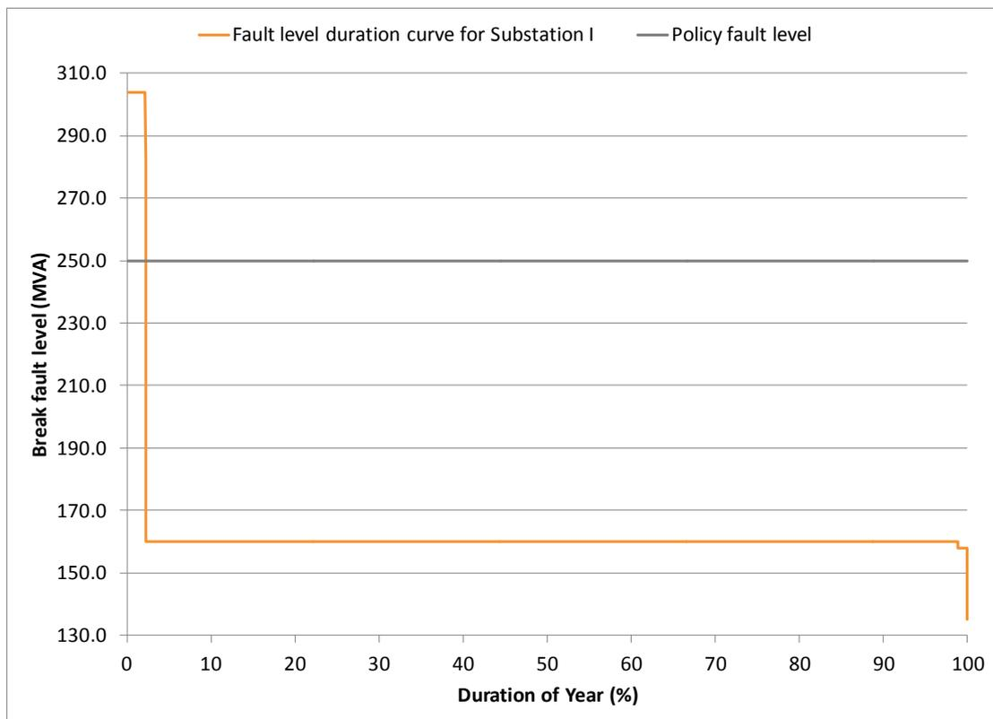
Figure D-27: Fault level duration curve for Substation I for the period 01 September 2012 to 31 August 2013
