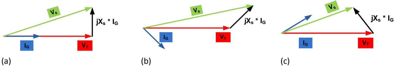
Figure 5-3: The vector calculation for generator internal voltage when it operates at (a) Unity power factor, (b) Lagging power factor, (c) Leading power factor
