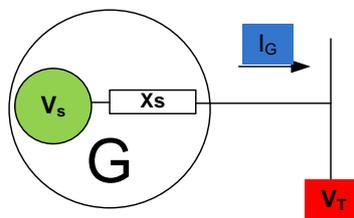
**Figure 5-2: Thevenin model of a generator connected to the network**
