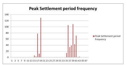
It can be seen that while the evening peak is still the dominant pattern there are many cases where the peak occurs in the morning confirming the results of the initial analysis. The Energy Model estimates for HV feeders dominated by industrial and commercial load are seen to tend peak during the day rather than in the evening.
