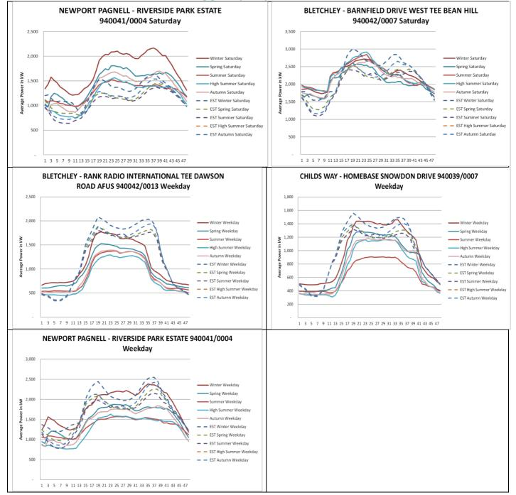
Sometimes the Energy Model underestimates the scale of the load. Given that it is more common to correctly estimate the scale for domestic feeders this suggests that a problem with the input data is more likely than a problem with the way in which the data is processed.
