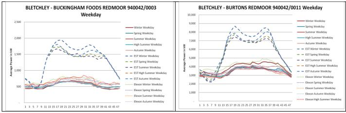
The Energy Model does not always reflect the impact that opening hours has on I&C loads.
