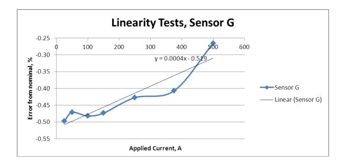
The results in Table 1b below indicate the departure from the linear fit for each sensor both in percentage of nominal applied current and in amps.
