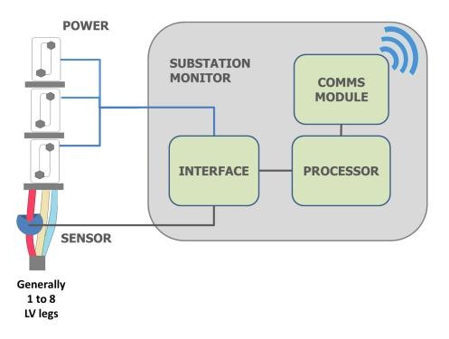
Figure 1: Fundamental components of a LV Substation Monitor.
