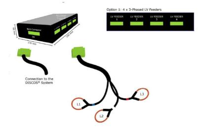
Figure 16: PowerSense LV satellite box and Rogowski coils
