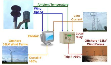
Dynamic Assets have previously being trialled and implemented on higher voltage circuits (33kV / 132kV) overhead line circuits to increase the output allowed from Wind Farms without having to replace or reinforce the connected circuits. Similar benefits could be obtained by expanding this technique to encompass points on the network where dynamic circuit ratings may be able to achieve extra utilisation within allowable rating.
