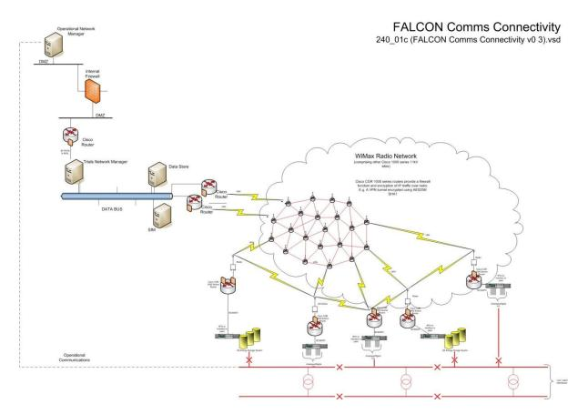
A pair of Cisco CGR1000 will be used to interface the network data to the Data Bus. This bus will connect the following:
