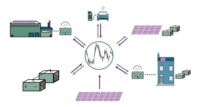
**Figure 1:** A DSO will use more real time data from smart technologies and services provided from different connected customers to help improve the management of the electricity network.
