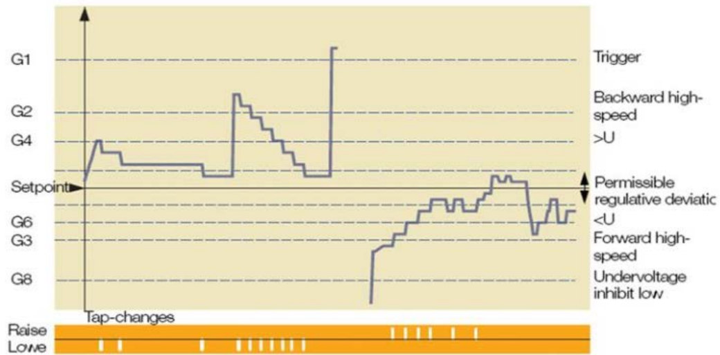
Figure 5-1: A-Eberle REG-D Hard Voltage Limit Capability
