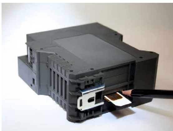
Figure 2-3 Inserting the SIM card
