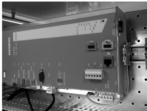
Master Control Module attached on DIN rail
