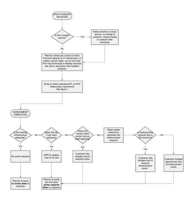
Figure 2 – WPD EV Charging Point Charging Methodology (EV rated > 32A)
