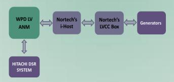
As shown, WPD's LV ANM system interfaces with Hitachi's DSR (developed as part of the Smart Energy Islands Project) in order to revise the generator curtailment based on the available DSR. The WPD LV ANM system then communicates with the generators through Nortech's i-Host and Low Voltage Connection Controller (LVCC) technologies. In the following weeks, the plan for the Factory Acceptance Testing (FAT) will be agreed and finalised, with the aim to complete the FAT in September.
